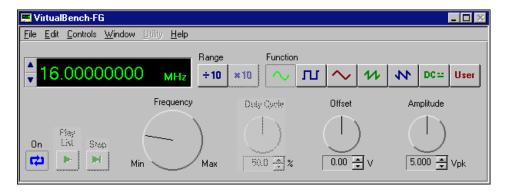
Figure 1-6. VirtualBench-FG Soft Front Panel for Function Generation
